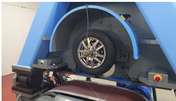
Fig.3 Tire testing machine used to measure tire characteristics
